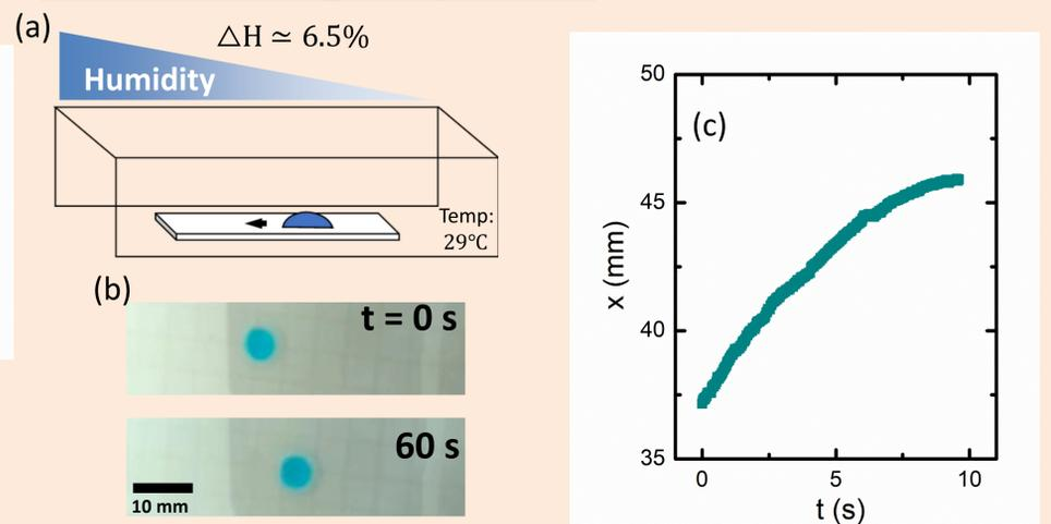
(a) A tunnel with a humidity gradient (6.5% R.H. at 29 °C) is constructed to test how the evaporation difference affects the droplet motion.
