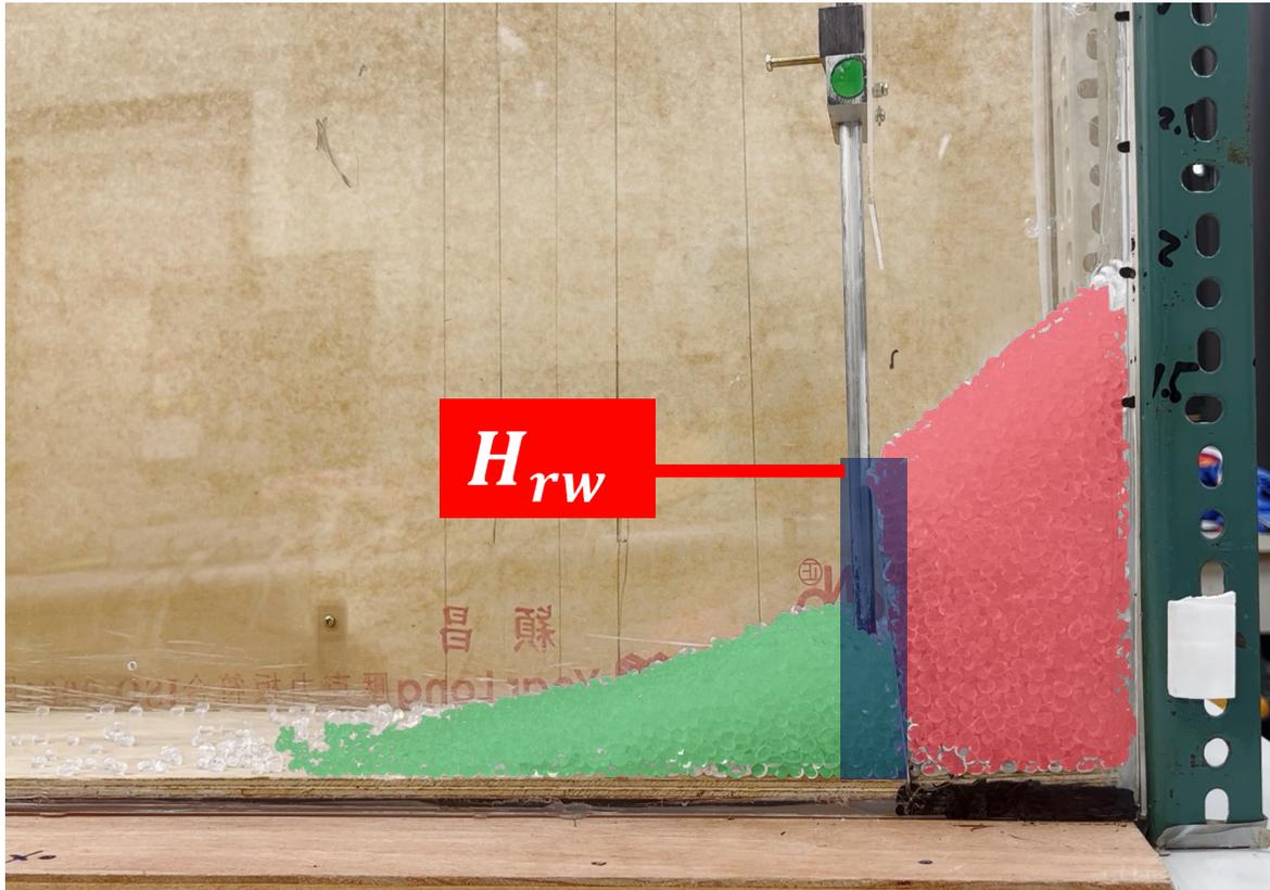
Calculate the loss ratio under different aspect ratios.
