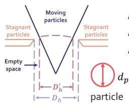
$D_h > 6d_p$ , the particles uninterrupted flow.
