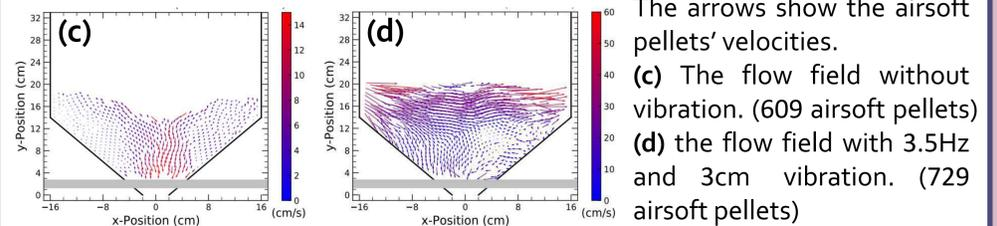
In (c), it shows the funnel flow. The airsoft pellets in the middle discharge first. In (d), it shows the inverted-funnel flow.
