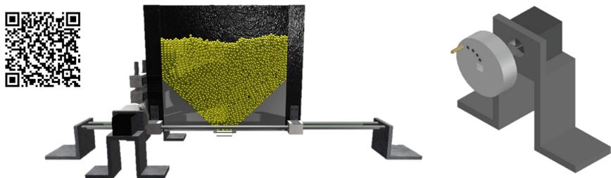
Using two stepper motors to push the hopper and changing the amplitudes by the holes in different locations. The details can be viewed by scanning the QR code.
