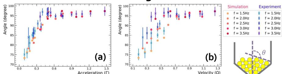
Change the different frequencies (1.5Hz, 2Hz, 2.5Hz, 3Hz, 3.5Hz) and different amplitudes (1cm, 1.5cm, 2cm, 2.5cm, 3cm), (a)  $\Gamma-\theta$ , (b)  $\Omega-\theta$
