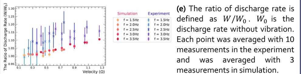
(e) The ratio of discharge rate is defined as  $W/W_0$ .  $W_0$  is the discharge rate without vibration. Each point was averaged with 10 measurements in the experiment and was averaged with 3 measurements in simulation.
